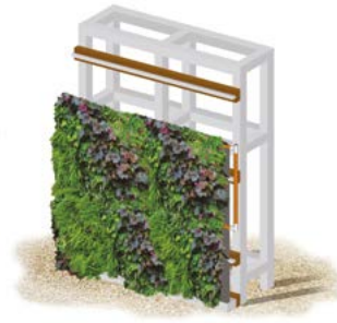
Install irrigation pipe on each row of modules
