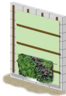
Install irrigation pipe on first row of modules
