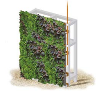
Finished wall connected to irrigation system.
